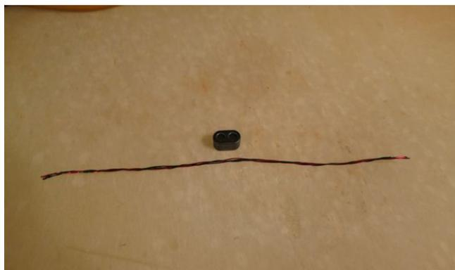
The end of this bundle that has the two loose crimped doubled ends is used to wind 4 turns through the core. I was careful to keep the windings adjacent as much as possible, not crossing over each other, to maximize the available space. A wood round pointed toothpick is useful to pack the windings to make space for the next pass. Be careful not to scrape the wire
